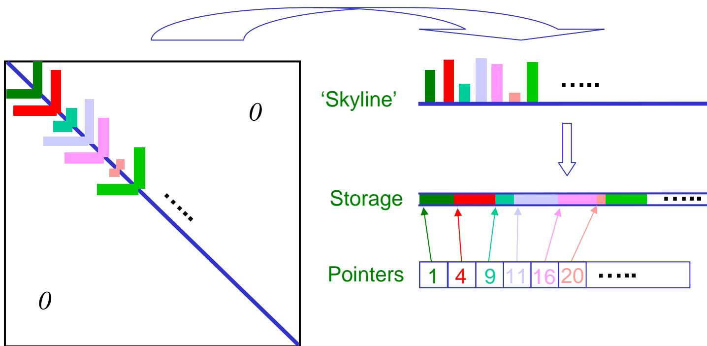
Skyline storage applicable when no pivoting is needed, e.g. for banded, symmetric, and positive definite matrices: FEM and FD methods. Skyline solvers are usually based on Choleski factorization
