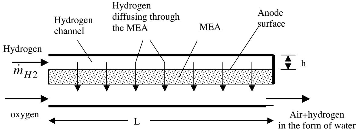
(i)  $h/L = 10^{-2}$  and  $Uh^2/(vL) \sim 0.025$ , the flow can be treated as locally fully developed.
