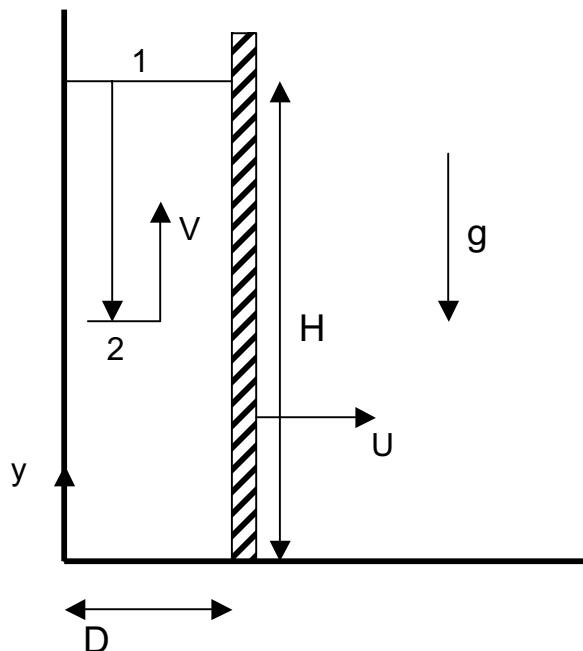
The flow is inviscid and incompressible. Since  $H \gg D$ , we make the approximations that it is one dimensional.
