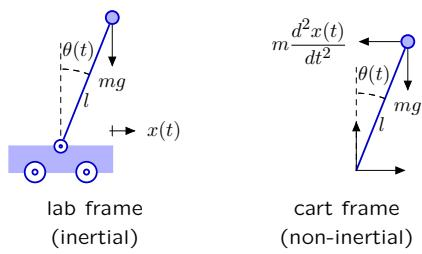
$$\underbrace{ml^2 \frac{d^2\theta(t)}{dt^2}}_I = \underbrace{\frac{mg}{l} \sin \theta(t)}_{\text{force}} - \underbrace{m \frac{d^2x(t)}{dt^2} l \cos \theta(t)}_{\text{force}}$$
