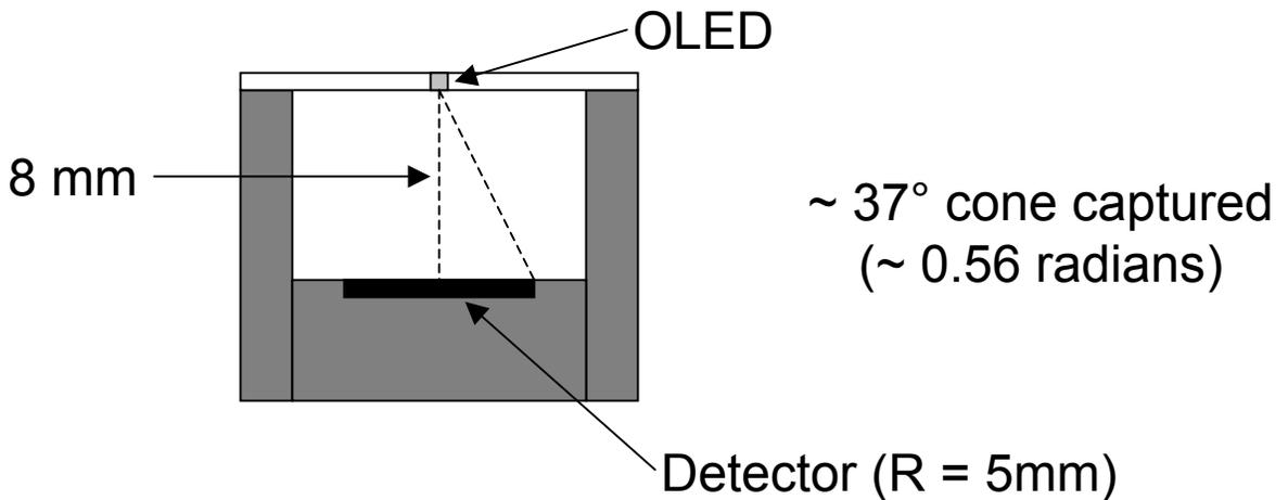
Output intensity profile from OLED:  $I(\Theta) \sim \cos^2 \Theta$
