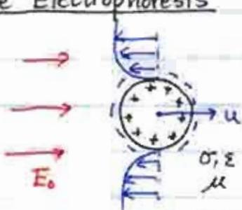
$$\left( \frac{u}{E_0} \right) = \frac{\left( \frac{\epsilon \sigma}{\mu} \right)}{1 + \left[ \left( \frac{\epsilon}{\sigma} \right) \left( \frac{\delta \sigma_m}{R \mu} \right) \right] + \left[ \begin{array}{l} \text{double layer} \\ \text{= surface conductivity} \end{array} \right] + \dots}$$
