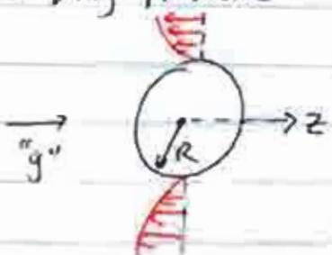
$F_{tot} = 0$  particle falling w/ constant velocity
