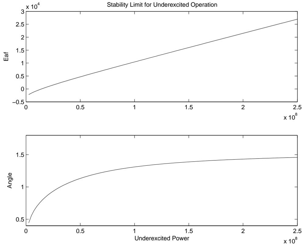
Figure 1: Angle and Field Current at Stability Limit
