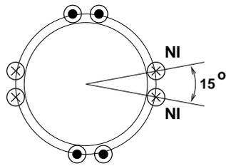
Figure 6:  $m=2$ , Full-Pitch Coil Arrangement
