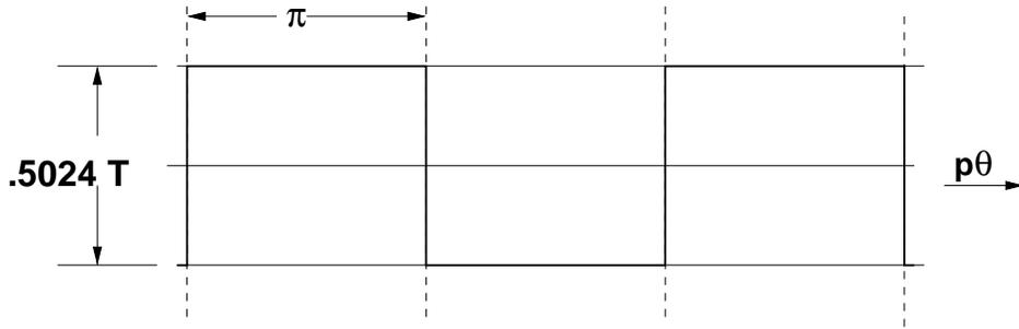
Figure 4: Full-Pitch Coil Flux Density
