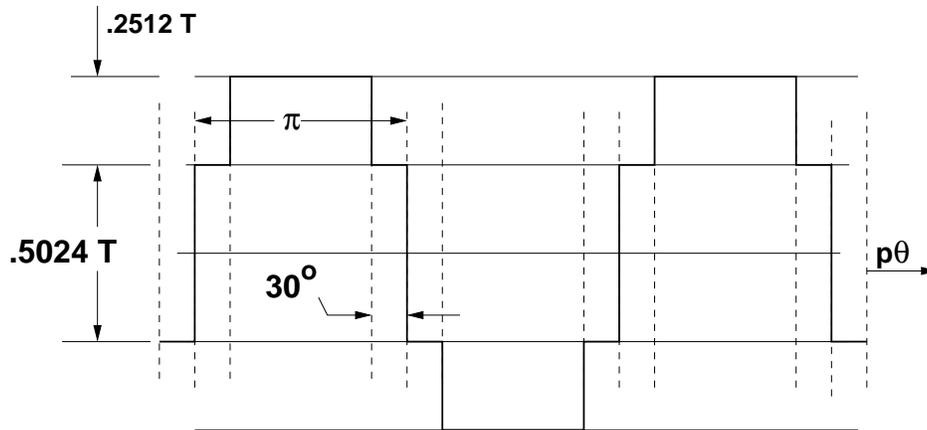
Figure 9: Flux Density from  $m=2$ , Short Pitch
