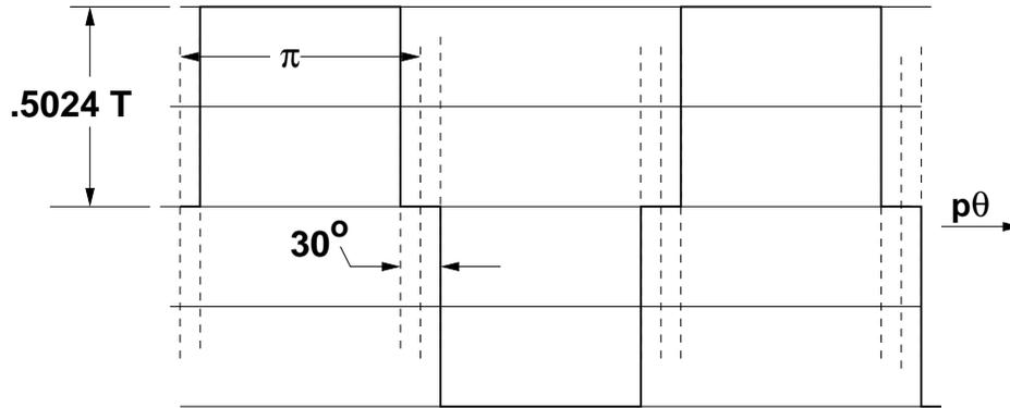
Figure 7: Flux Density from  $m=2$ , Full Pitch
