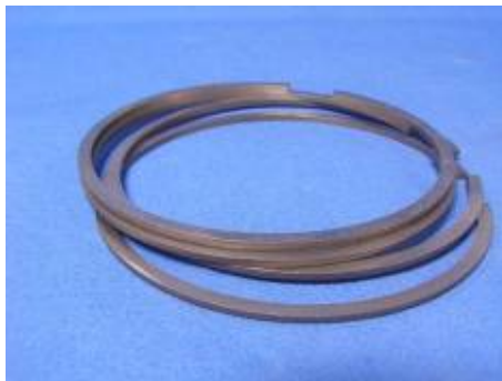
Figure 19. Prototype E2: 77 (Ti,Mo) (C,N)–20Ni–3 Mo
