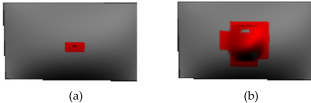
Figure 18. Feature extracted, at resolution level 5, on artificial curved mesh with a) small dent, and b) large ding.
