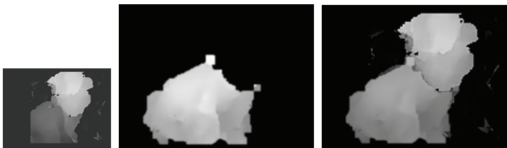
Fig. 6. (a)disparity map generated from 160x120 stereo images, (b) from 320x240 stereo images, (c)Composition of above disparity maps
