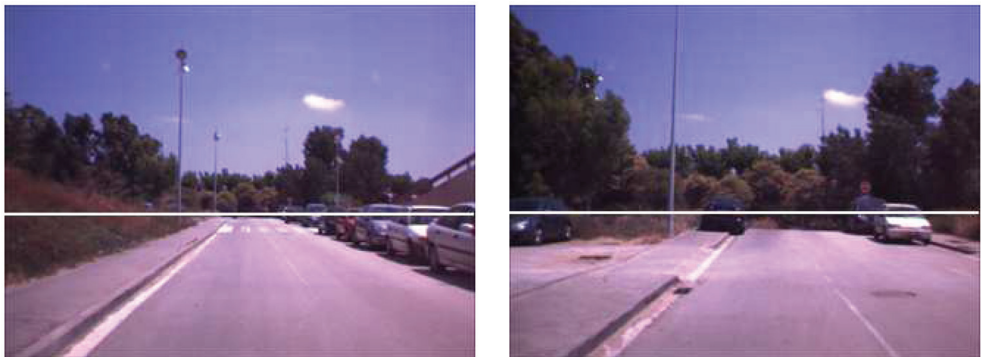
Fig. 7. The estimated horizon line associated with frames 10 and 199. The sequence corresponds to an uphill driving.
