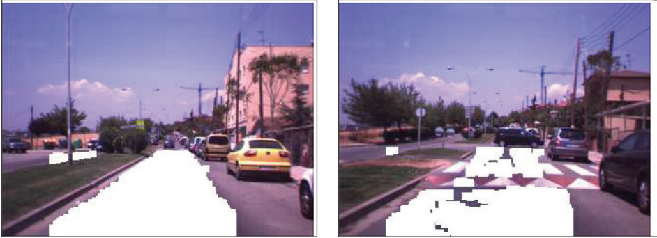
Fig. 3. Rapid road segmentation associated with two frames.
