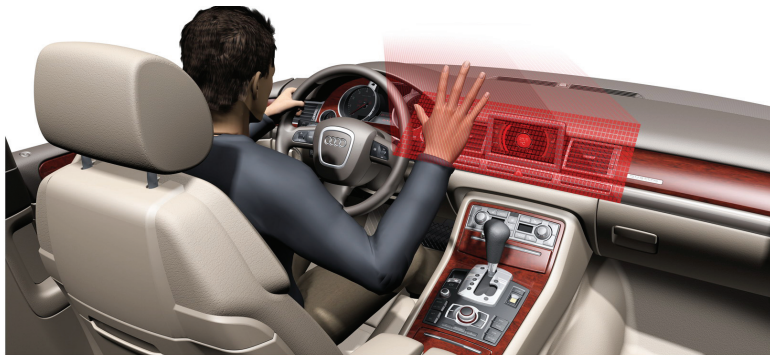
Fig. 4. Smart airbag application using a PMD TOF vision systems (Husmann & Hess, 2006)
