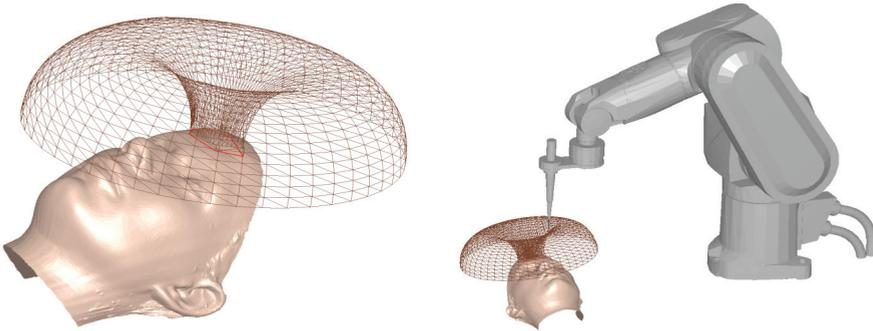
Fig. 5. Detail of a virtual shield and the scenario including the robot arm.
