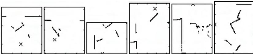
Figure 8. 6 out of 60 scans of the NIST rescue scenario data set. The scans in this data set are very sparse and have minimal overlap
