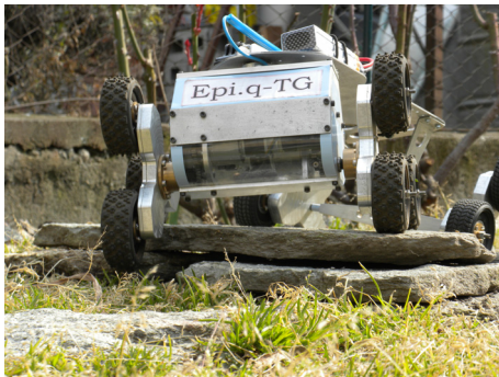
Fig. 17. Epi.q-2 traversing an obstacle, on uneven ground
