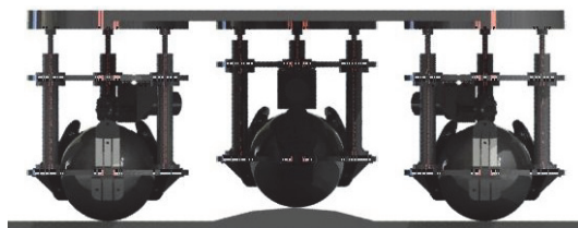
Fig. 5. Wheels adjustment with obstacle owing to proper action of suspension system.
