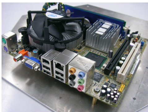
Fig. 14. PC based controller and Solid State Disk (SSD)
