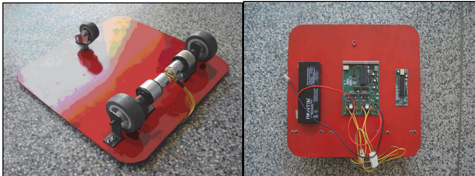
Fig. 24. The mechanical structure of the Emmy III second prototype
