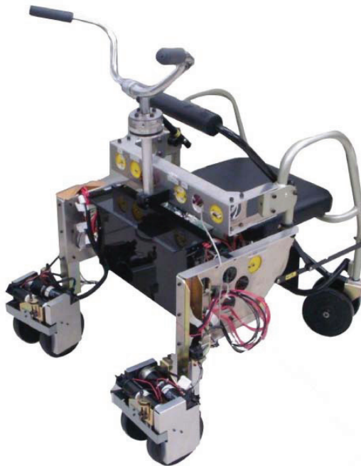
Fig. 1. The omnidirectional mobile robot in developing for the elderly's walking support, the disabled's walking rehabilitation, and the caregiver's power assistance
