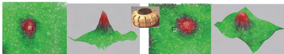
Fig. 24. Nonlinear images of AP mine VS-50 buried in gravel at 12 mm (left), NDC =19dB, and 25 mm (right), NDC =16dB
