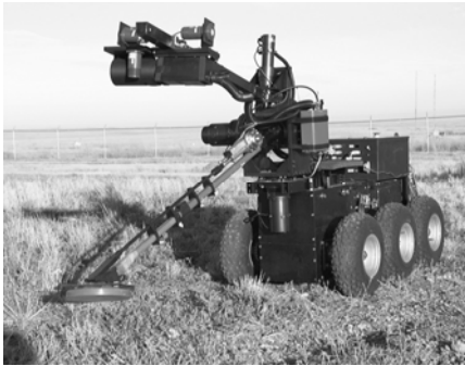
Fig. 5. Robotic Scanner mounted on teleoperated vehicle[5]
