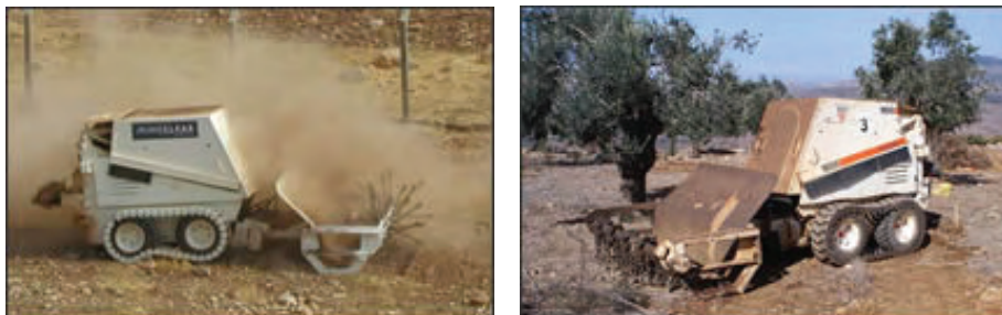
Fig. 2. The mini-flail vehicles "Božena 2 and 3"
