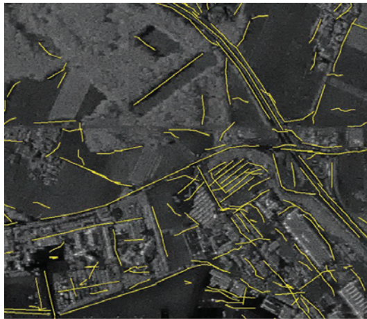
Fig. 7. Detection of lines in a full polarimetric L-band SAR image.
