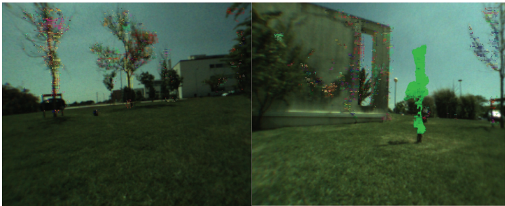
Fig. 7. A typical result of obstacle detection with the stereo head
