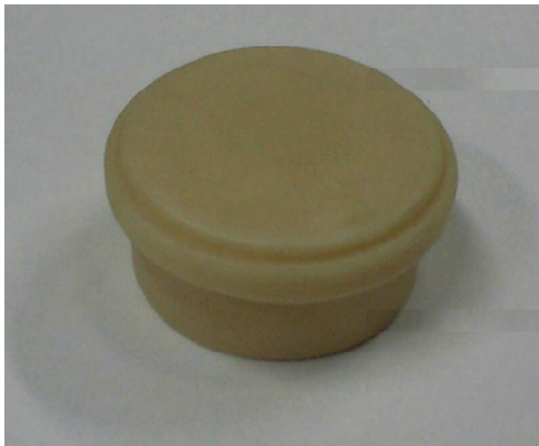
Fig. 8. Buried object: plastic case of a landmine shape
