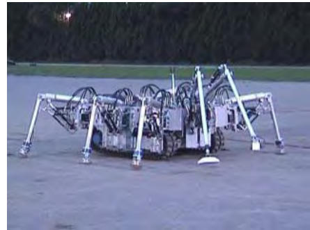
Fig. 4. Mine detection robot COMET-III
