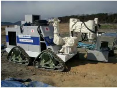
Fig. 7. Mine Hunter Vehicle with two manipulator
