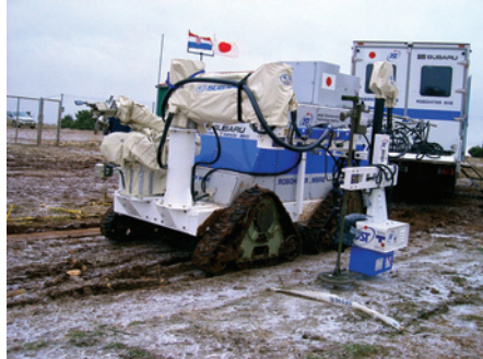
(b) SAR-GPR in operation in CROMAC test site. SAR-GPR scans in the side of MHV
