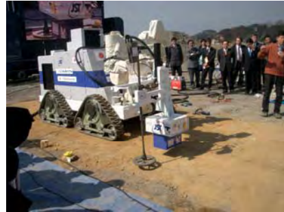
Fig. 8. Mine detection test of MHV
