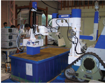
(a) SAR-GPR mounted on a robotic arm and scans in front of the MHV.
