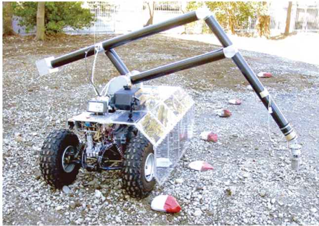
Fig. 3. Field Arm mounted on top of the mobile platform
