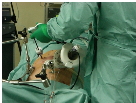
Fig. 3. View of an in vivo experiment (laparoscopic cholecystectomy) using a living swine. The P-arm and its supporting arm were so small that they did not interfere with the surgeon's work.
