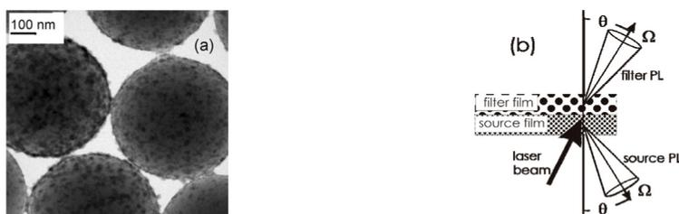
Fig. 21. (a) TEM image of 420 nm PS beads, which are LbL-coated by CdTe NCs in one deposition circle. The NCs appear darker due to the higher contrast. (b) Layout of the PL measurements.  $\theta$  - the angle of incidence and the angle of detection,  $\Omega$  - the solid angle of the light collection.
