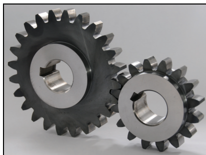
Fig. 15. Coated test gears used for testing pitting – type C-PT
