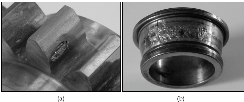
Fig. 2. The pitting wear: a) on a pinion gear, b) on a bearing race
