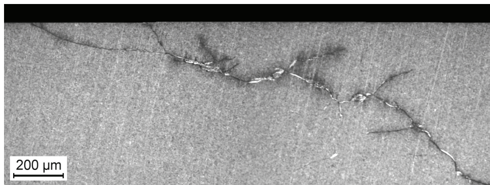
Fig. 52. LOM micrograph of the etched radial microsection of the case hardened inner ring of a CARB bearing from a paper making machine. The overrolling direction is left-to-right
