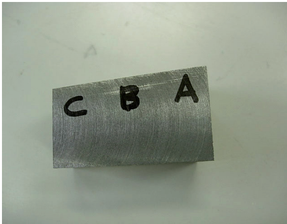
Figure 14. Three measuring points of a specimen (A: largest, B: middle, C: smallest in thickness).
