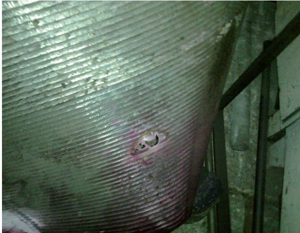
Figure 52. Position of the bubble open defect and of pores and oxides.
