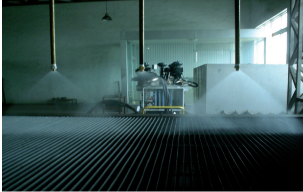
Figure 14. Experimental device of cold characteristics test for cooling nozzles
