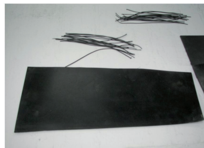
(b) convex section cutting from hard rubber
