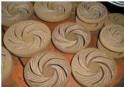
Figure 10. Examples of sand core which have rubber non-smooth structures pasted on their surface.
