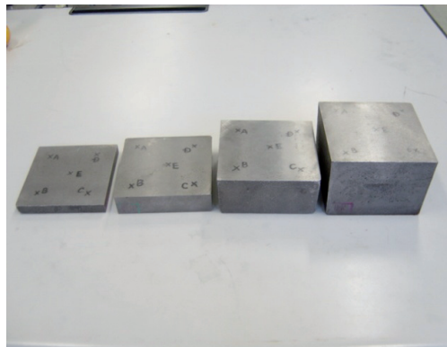
Figure 10. The specimens with three kinds of surface conditions (as-cast, machined and shot-blasted: 100 mm square, continuously cast bar).
