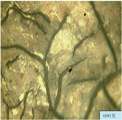
Figure 52. Flake graphite in a pearlitic matrix adjacent to the core in a hollow cylindrical casting.
