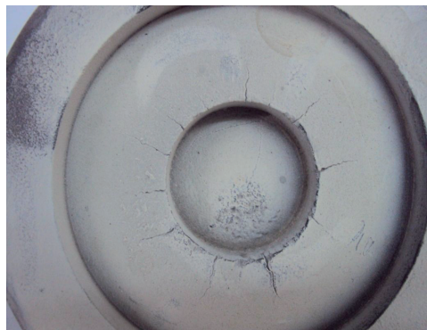
Figure 48. Typical Thermal Fatigue Cracks in a PM.
