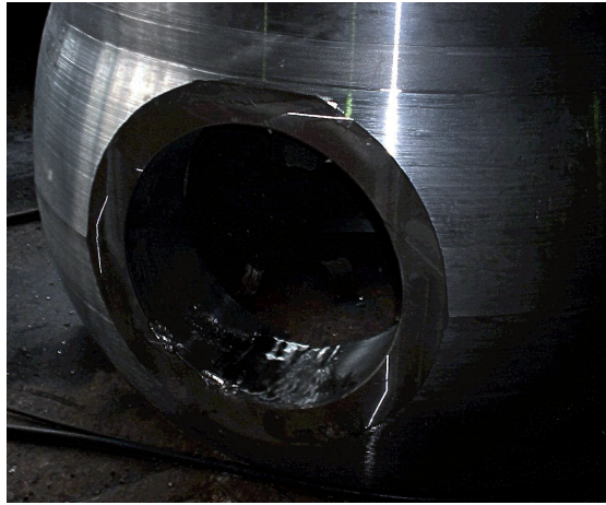
Figure 30. Casting defects in the block window.
