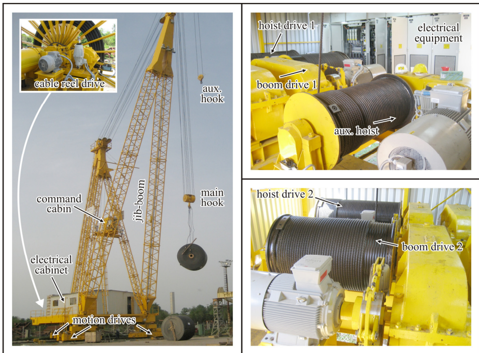
Fig. 13. Derrick crane with indicated drives.
