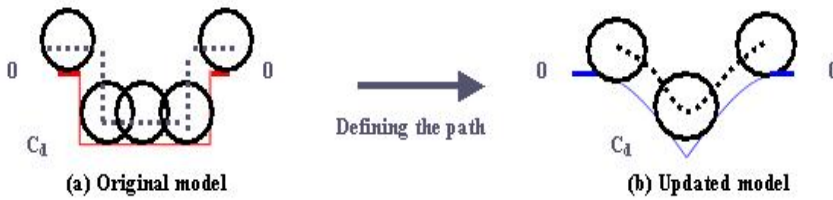
Fig. 3.4.2. Modified model of a spall based on a more realistic ball trajectory. [66]
