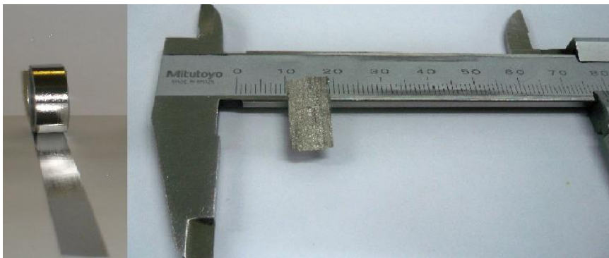
Fig. 13. \text{Fe}_{78}\text{Si}_{13}\text{B}_9 amorphous strips used in magnetic cores, and industrial magnetic package.
