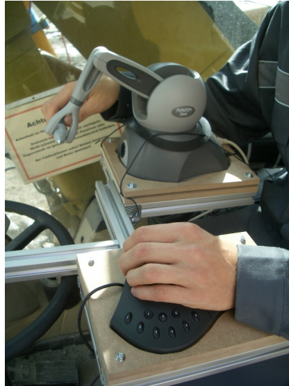
Fig. 5. Test excavator equipped with operating devices
