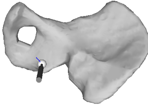
Fig. 12. A burr-tool receiving force-feedback from a polygonized pelvis model where the force (direction and strength) is displayed with a blue line
