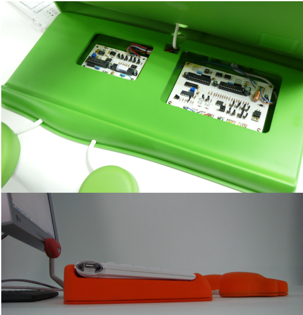
Fig. 10. Controller circuits underneath the keyboard base
