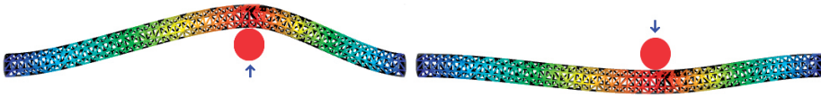
Fig. 4. Two deformations of the object for the identical position of the probe (depicted by the filled red circle) showing the non-flatness of the probe interaction model. On the left, the probe comes from the space below the deformable body, on the right it comes from the space above the body (the directions are depicted by the blue arrows).
