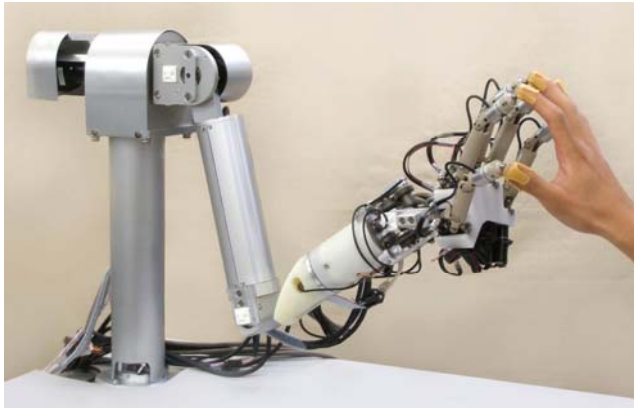
Fig. 1. The Developed five-finger haptic interface: HIRO II
