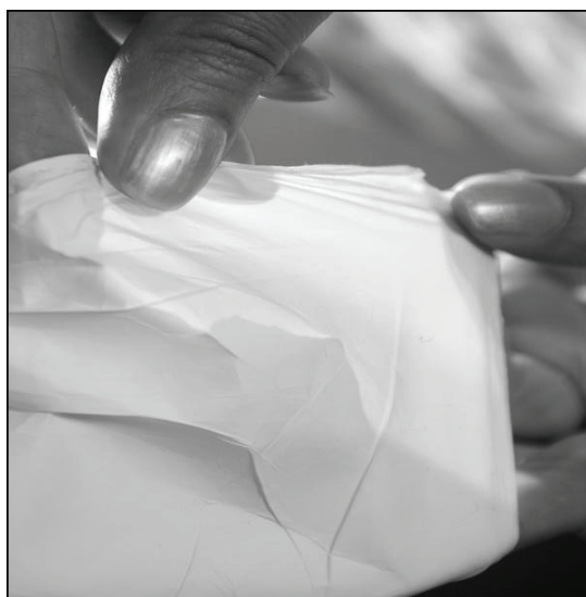
Fig. 2. (a) Basic apparatus for electrospinning, (b) A photo of typical electrospun nanofibre mat.
