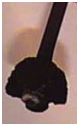
Fig. 6. Carbonaceous depot in cathode, when dc current is used
