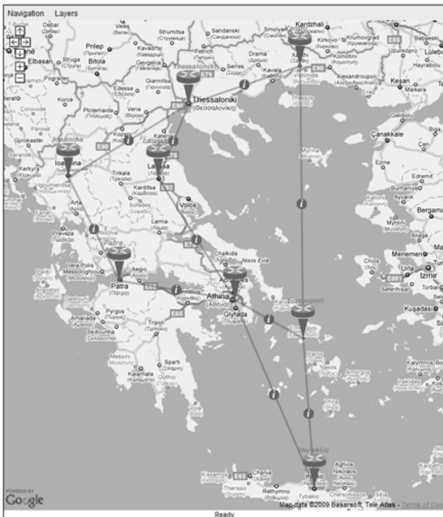
Fig. 1. GRNET's Layer 3 Country Network Topology
