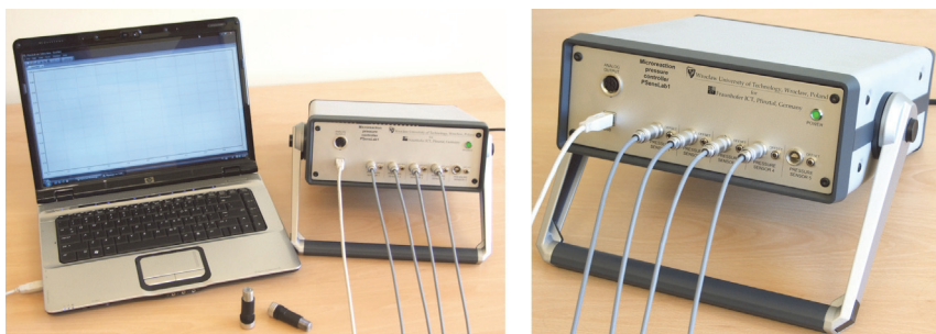
Fig. 16. Commercial-like measurement system driving 5 discrete pressure sensors
