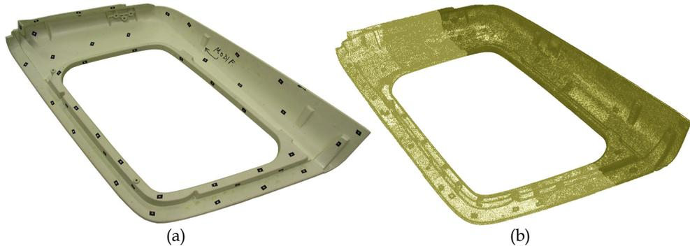
Fig. 15. (a) Physical model; (b) final polygonal model of the door chassis
