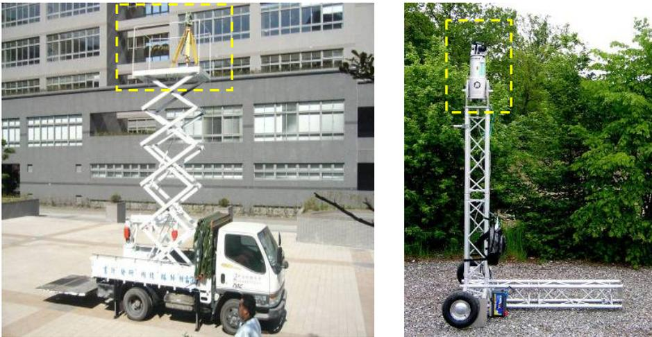
Fig. 4. lift-able car and movable support
