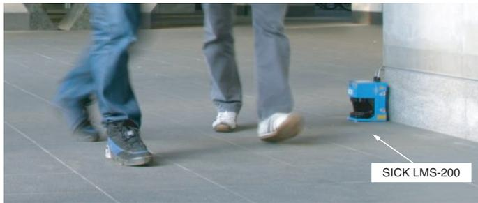
Fig. 2. Snapshot of human sensing using a laser scanner
