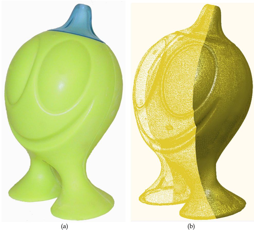
Fig. 11. (a) Physical model; (b) final polygonal model of the sugar bowl
