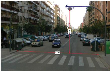
(a) Laser Scanner Positioning
