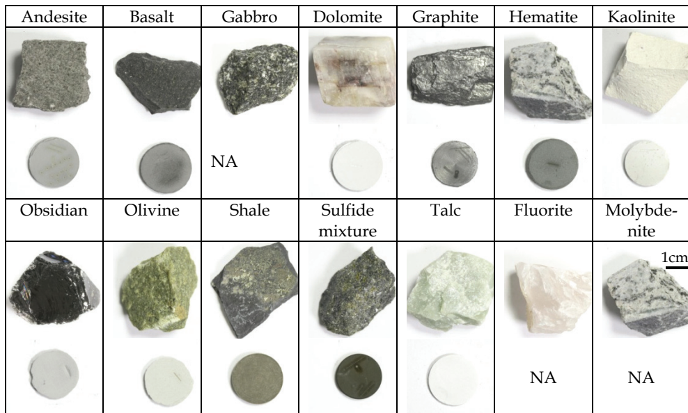
Fig. 7. Natural rock & mineral samples and their powder tablets counterparts.
