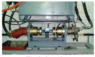
Fig. 12. Bosch servo motor, type EP2, within the secondary sector
