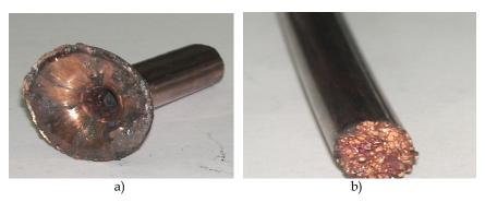
Fig. 3.8. The flow-through flaw on after end (a) and loosening on exposed face (b) of samples obtained from fibrous pressing
