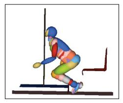
Fig. 24. 235 ms: the neck reaches the critical position: this is the maximum deflection
