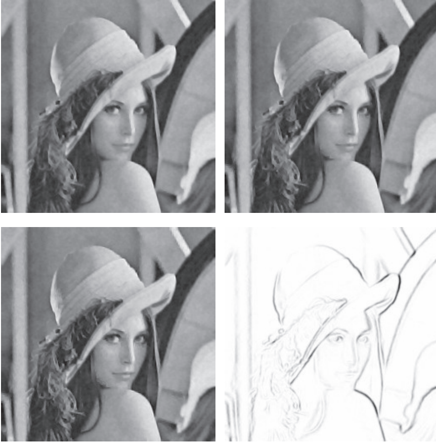
Fig. 4. Image restoration with the continuous TD algorithm R_{D_T} -Continuous (Aniso) for the Lena image with k_0 = 2 , upper row: \alpha = 0.10, 0.20 , lower row: \alpha = 0.30 and TD value for each pixel.
