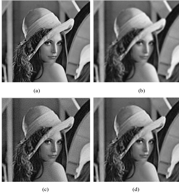
Fig. 25. (a) Original Image, (b) Blurred Image, (c) After Projected Landweber, (d) After twPIT
