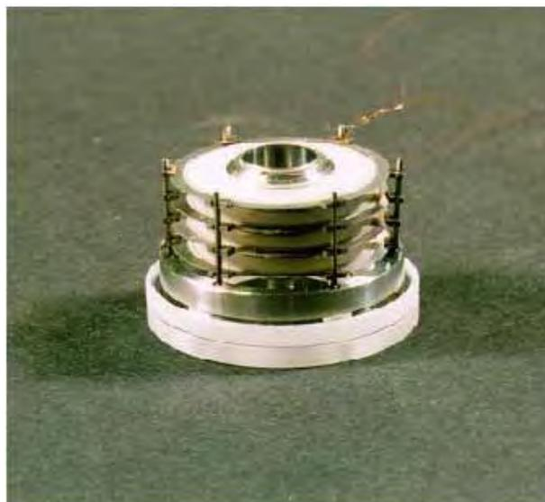
Figure 7. Dynamic Focusing Lens
