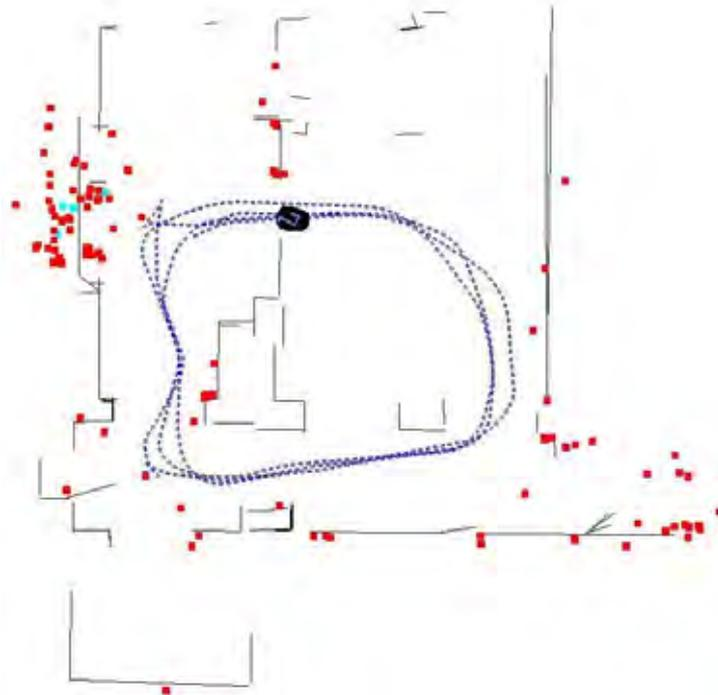
Figure 5. The landmark map with the trajectory and reference laser based map
