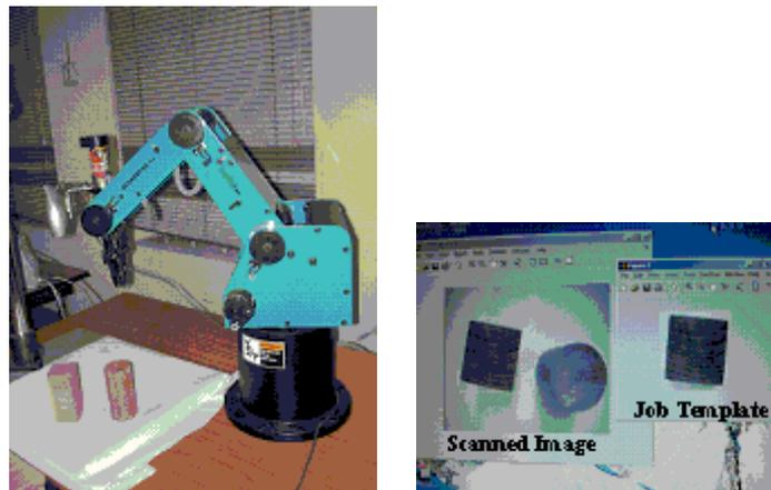
Figure 4. Manipulator setup for material handling using template matching
