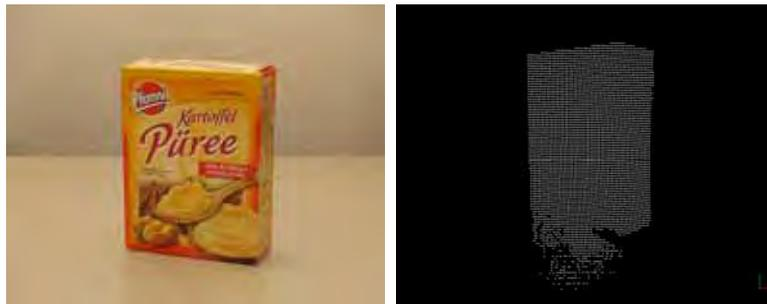
Figure 13. An instant mashed potatoes box. Because of the symmetry plains of the cuboid shape the pose determination gives a set of possible poses. Left: Colour image from a digital camera. Right: 3D range image from the Swissranger SR-2
