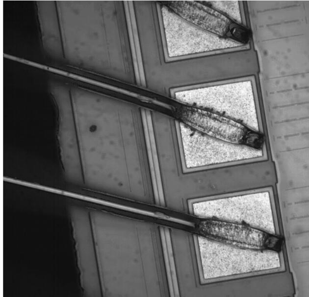
Figure 23. Example of All-in-Focus Image about wire bounding
