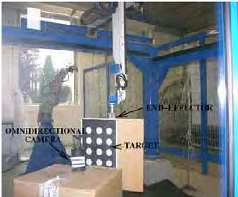
Figure 6. Experimental setup : eye-to-hand configuration
