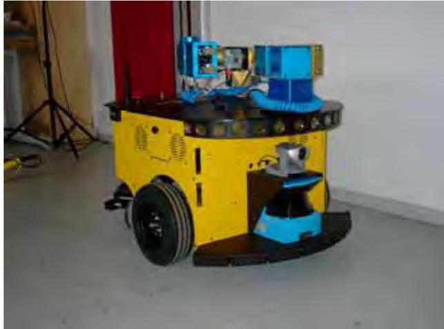
Figure 4. The PowerBot platform with the Canon VC-C4 camera
