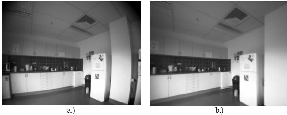
Figure 7. An image from a wide angle lens. a.) raw. b.) rectified
