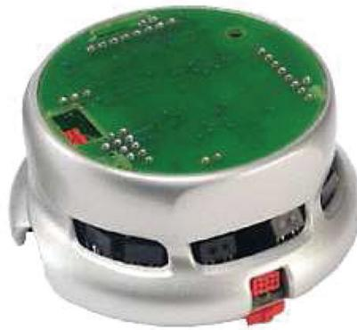
Fig. 2. The miniature mobile robot: Khepera
