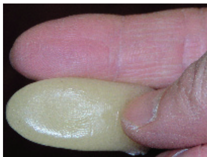
Fig. 3. Dummy fingerprint made by kitchen powder.
