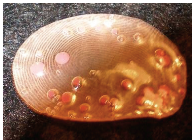
Fig. 2. Dummy fingerprint made by polymer.
