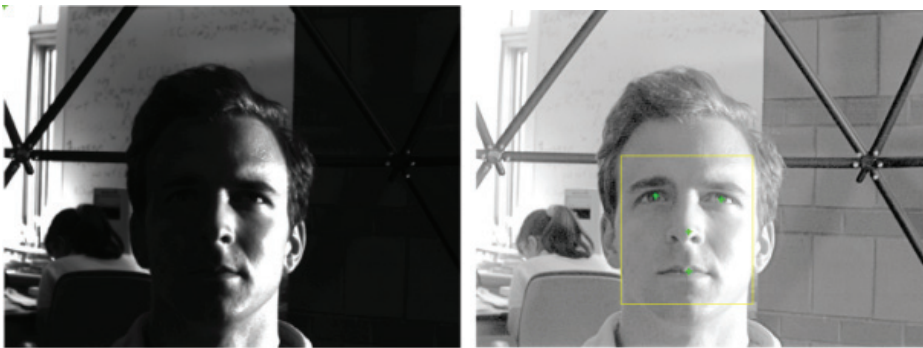
(a) Without preprocessing, face detector does not work (b) With preprocessing, face detector works well
