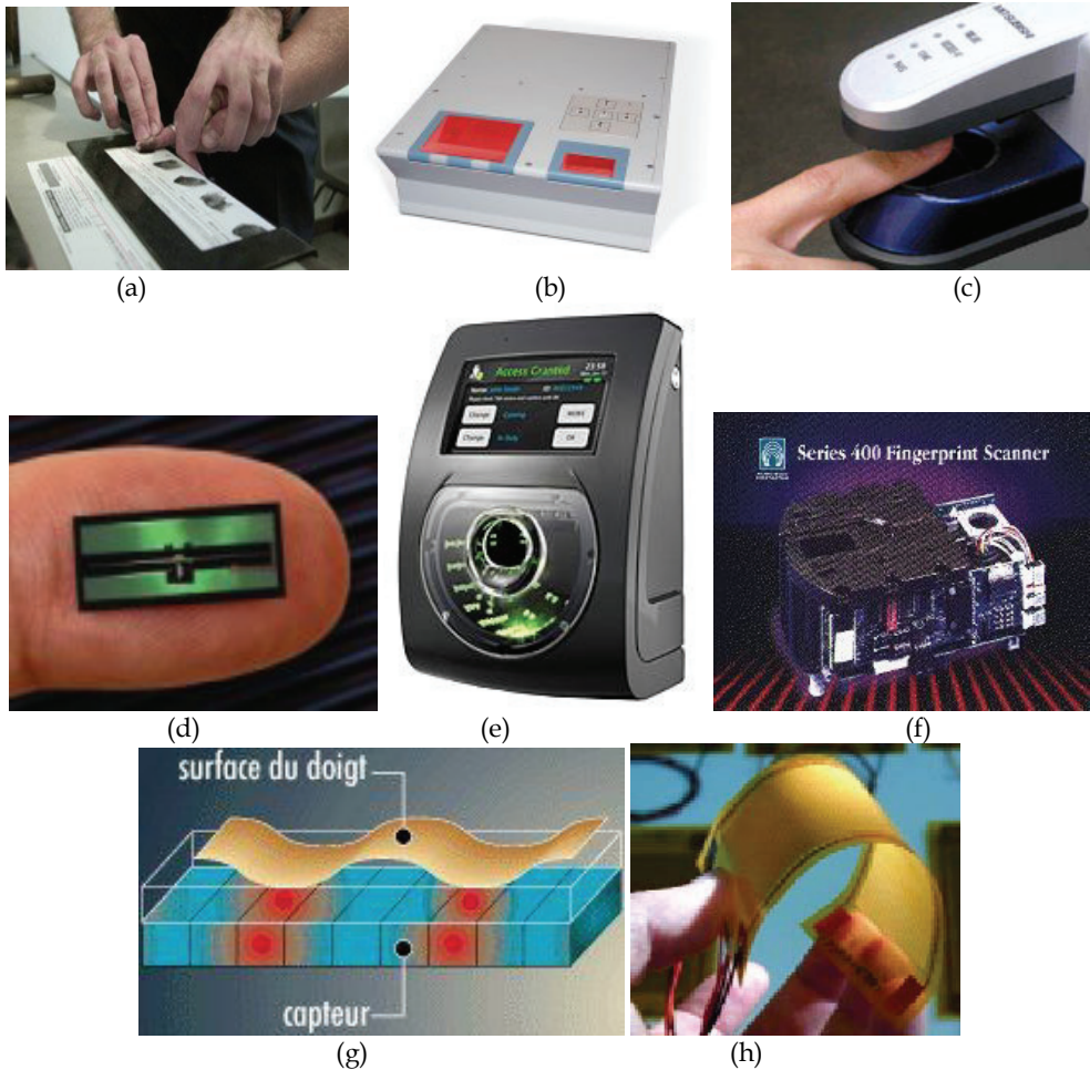
Fig. 1. The development of fingerprint acquisition devices, (a) ink (b) optical rolling devices (c) regular camera for fingerprint scan (d) silicon-capacitive scanner (e) optical touchless scanner (f) ultra sound scanner (g) thermal sensor (h) Piezo-electric material for pressure sensor
