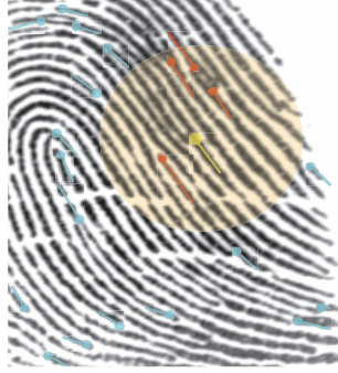
Fig. 12. The \delta -neighbourhood ( \delta = 4 ) for a given minutia (ignoring false crease minutiae).
