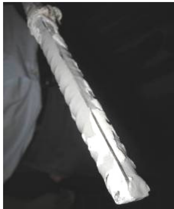
Fig. 19. Interlocking surface in an anchor installed into a hole which is not filled with epoxy (Photo by Dr. Halil Nohutcu)
