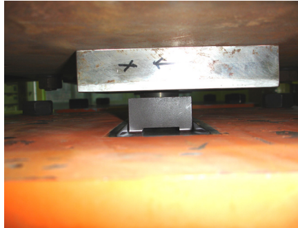
Fig. 21(b). Slider located between the concave trench and the spherical concave surface.
