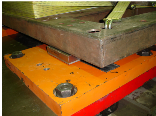
Fig. 20(a). Assembly of direction optimized friction pendulum system
